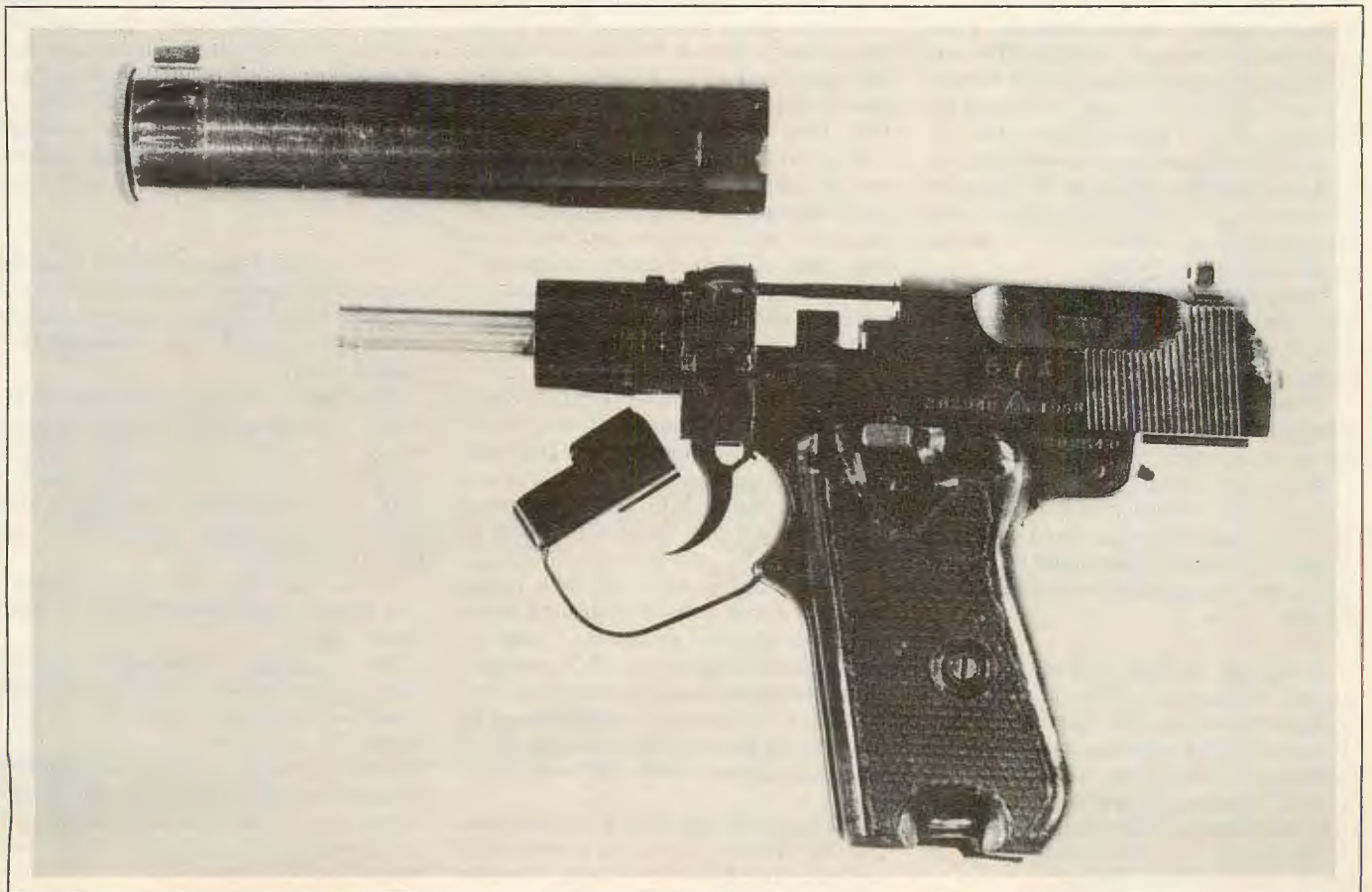
Model 67 with silencer removed, slide back and trigger guard lowered on hinge. Note slimness of barrel.
